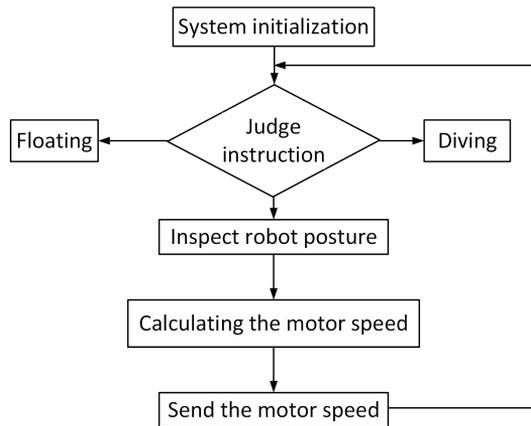
Fig. 3. The software design process of the Robot attitude control system
